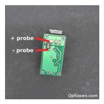
We recommend to check/set the current using a test load resistor because it is much safer and will limit the possibilities of mistake.
